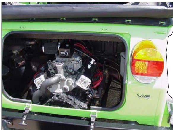
Colin's 1992 3.1L Chevy Lumina V6 Short Block
